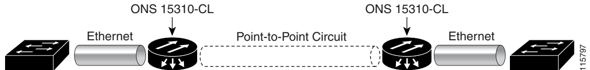
Figure 17-1 CE-100T-8 Point-to-Point Circuit
